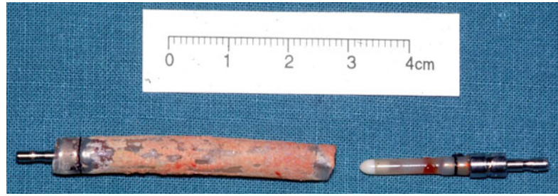
Fig. 8.4 Shunt valve of Holter type, removed during shunt revision, 20 years after implantation. The valve case has completely disintegrated due to material destruction. Extensive calcification is seen on the outer surface
