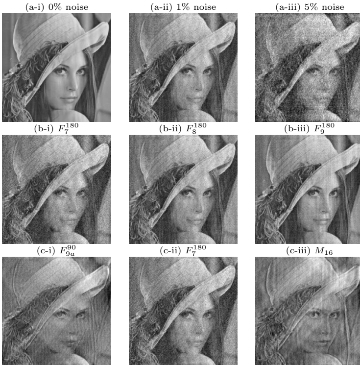
Fig. 5. (a) Reconstruction using MFI for Mojette data with angle set F_8^{180} . Amount of Gaussian noise added as indicated. RMSE (i) 6.0 (ii) 16.2 (iii) 26.7. (b) Reconstruction using MFI for Mojette data with 1% Gaussian noise added using angle set as indicated. RMSE (i) 19.5 (ii) 16.2 (iii) 13.1. (c) Reconstruction using MFI for Mojette data with 1% Gaussian noise added using angle set as indicated. RMSE (i) 28.3 (ii) 19.5 (iii) 29.1.
