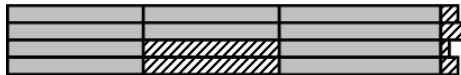
Fig. 2. A layer with 6 bars of length L_1 and 4 bars of length L_2 . Scrap is marked with a slanted pattern.
