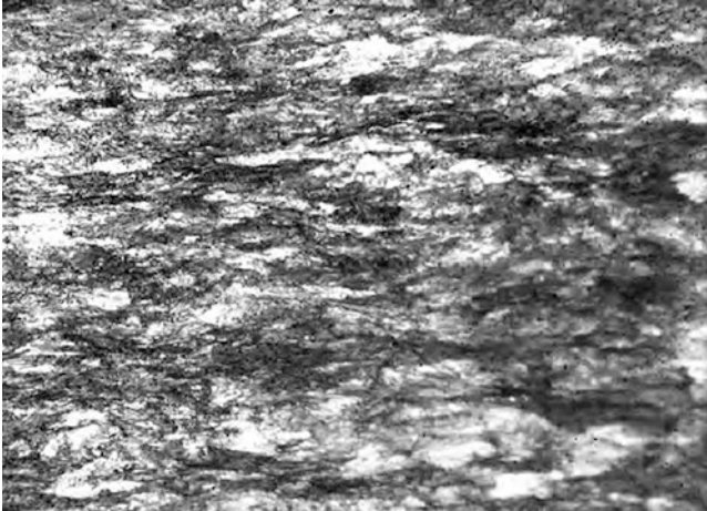
Fig. 1 Micrography \times 500 (500 increments) longitudinal section of cold drawn steel
