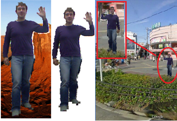
Fig. 5. The user is segmented from the background and then displayed in the program. The Kinect image is mirrored, so we reverse this to preserve the correct image.
