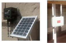
Fig. 2. Civitas pollution monitoring node (left) and service node (right) deployed in the school of computer science
