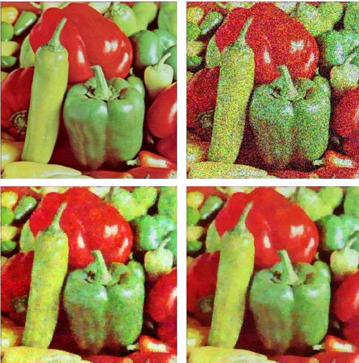
Fig. 6. Example of the image denoising results for Peppers (from left to right and top to bottom, the original image, the noisy version and the recovery images using TV and GTV)
