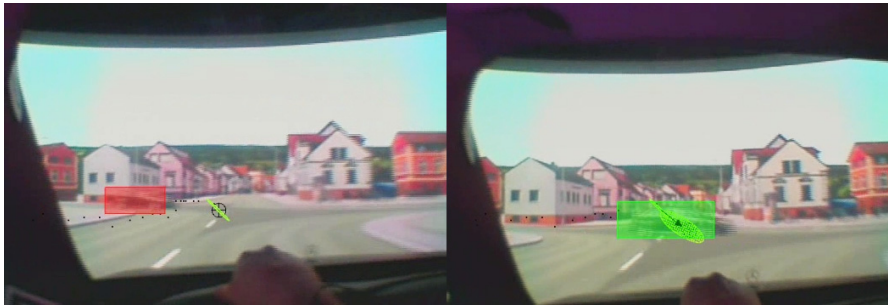
Fig. 6 A car appears on the left of the driving scene and is about to cut the driver’s way. The red bounding box around the approaching hazard and the driver’s fixation cluster are shown. Once the bounding box is intersected by the fixation cluster, the traffic hazard is marked as “perceived”, highlighted by the green bounding box [TKK + 13].
