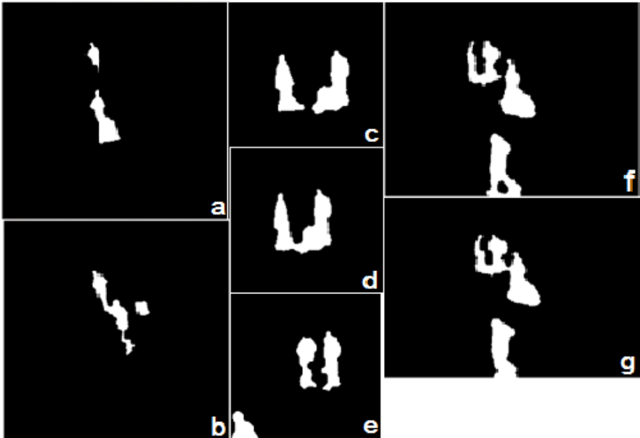
Fig. 1. (a) Two separate masks (one belongs to a person, the other one belongs to a person with a package). (b) Two separate masks (one belongs to two people, the other one belongs to a person with a package). (c) Two separate masks (one belongs to a person, the other one belongs to a person with a package). (d) One mask (two persons and a package). (e) Three masks (each belong to a person). (f) Three masks (one belongs to two persons, the other one belongs to a person and a package, the third one belongs to a person). (g) Two masks (one belongs to three people and the other one belongs to a person).
