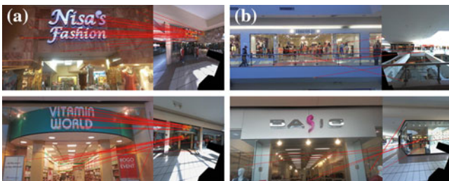
Fig. 5.11 a Successful and b unsuccessful examples of image retrieval. Red lines show SIFT feature matches
