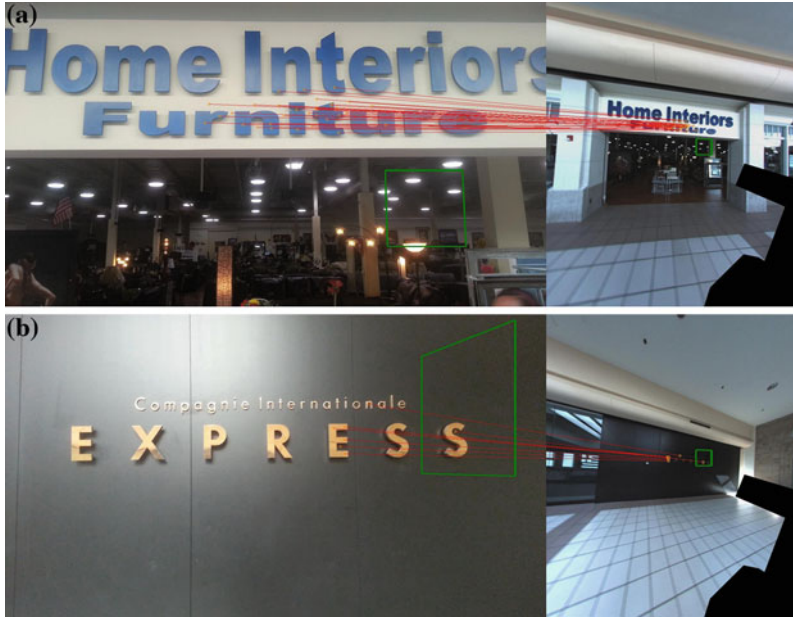
Fig. 5.13 a Example of accurate pose estimation on query image. b Example of inaccurate pose estimation. Notice how different letters in the same sign are matched
