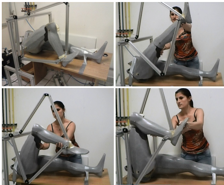
Fig. 6 Mechanism performing rehabilitation motions with a mannequin
