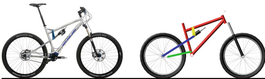
Fig. 2 A picture of the bicycle and the multibody model of the bicycle ( left is courtesy of Meissner Raeder)
