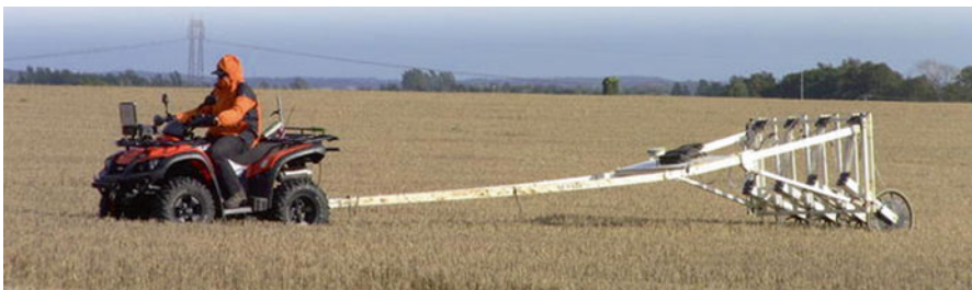
Fig. 5.1 Motorized magnetometer prospection at the Iron Age site of Uppåkra in southern Sweden using a multichannel Foerster gradiometer array mounted on a nonmagnetic cart (Image courtesy of Ludwig Boltzmann Institute for Archaeological Prospection and Virtual Archaeology)
