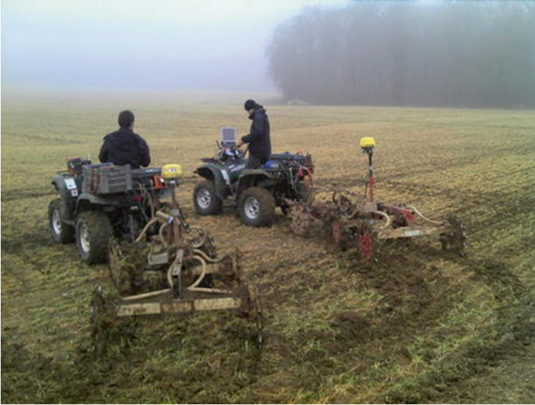
Fig. 5.3 Automatic Resistivity Profiling with two ARP(c) systems. The electrodes are the toothed wheels (Image courtesy of Geocarta, Paris)
