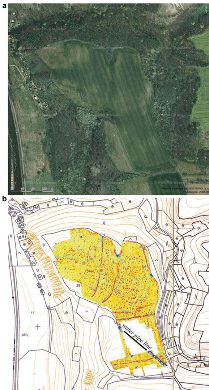
Fig. 27.1 Zlončice, district Mělník. Combination of (a) vertical aerial photography (public web source www.mapy.cz ) and (b) the result of magnetometric survey of prehistoric hillfort (terrain: plowed field and meadow; surveyed area: approx. 9.5 ha; magnetometric survey: Křivánek 2008–2010)
