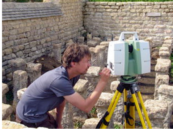
Fig. 7.2 Laser scanning carried out by the University of Birmingham at Chedworth Roman Villa, Gloucestershire (UK), on behalf of the National Trust (Photo: Jason Wood)
