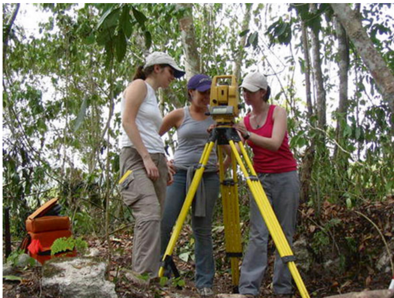
Fig. 17.1 Undergraduate students Alex Miller, Shelley Khan, and Yasmine Baktash ( left to right ) set up a Topcon GTS 605 laser theodolite to digitally map Chan's settlement (Photograph by James Meierhoff)
