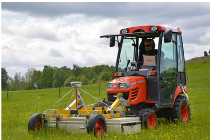
Fig. 5.5 Motorized GPR survey with the 16-channel MALÅ Imaging Radar Array at the UNESCO World Cultural Heritage site Birka-Hovgården. Data positioning is conducted with the GPS antenna mounted on top of the GPR system (Image courtesy of Ludwig Boltzmann Institute for Archaeological Prospection and Virtual Archaeology)
