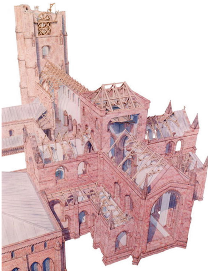
Fig. 7.6 A cutaway reconstruction drawing of the church at Furness Abbey, Cumbria (UK) (Drawing: David P Cooper)
