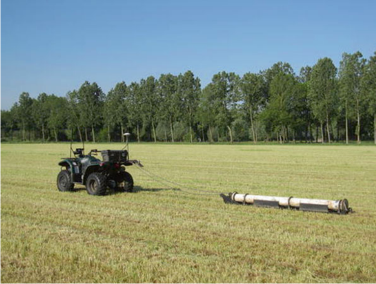
Fig. 5.4 The DUALEM-21S sensor for simultaneous measurement of apparent resistivity and magnetic susceptibility mounted in a sled, pulled by an all terrain vehicle with DGPS and Lightbar Guidance System (Image courtesy of Wim De Clercq, Gent University)
