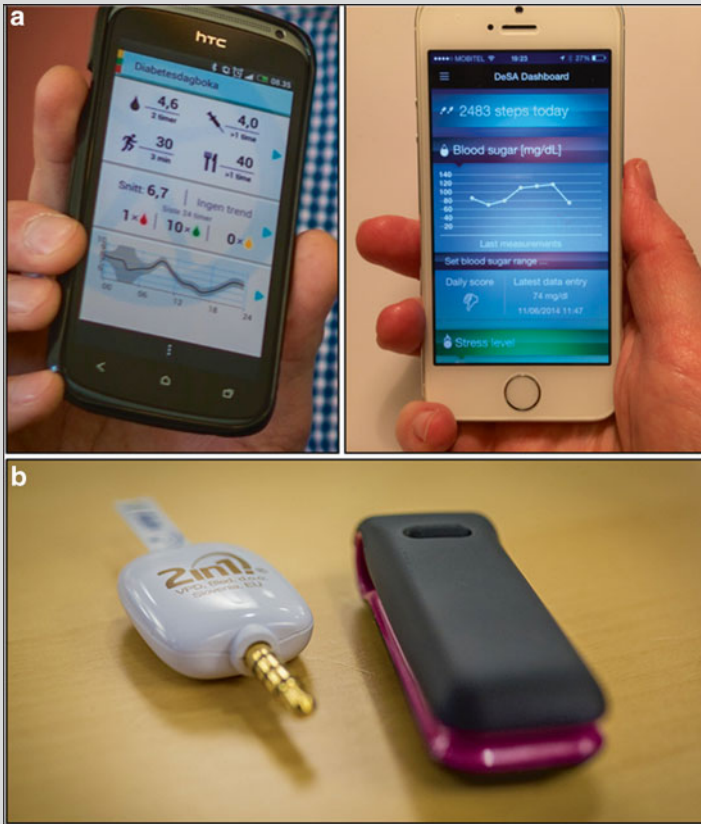
Fig. 8.7 Case study: (a) The Diabetes Diary smartphone app (left), the DeStress Assistant smartphone app (right), (b) 2in1SMART glucometer (left), and FitBit physical activity monitor (right)
