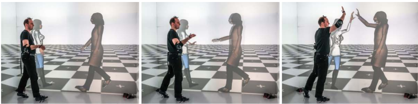
Fig. 5. The virtual agent’s postures are optimized for live human agent interactions. In this example a user high fives a virtual character successfully. The agent adopts its motion to meet the users hand at the right time and position.
