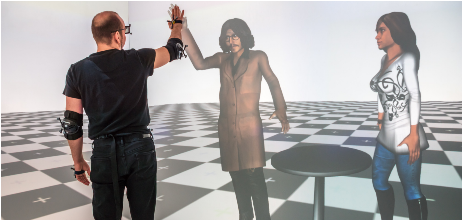
Fig. 1. A virtual agent’s animation is calculated based on live human motion data. For that we first analyze the user’s current and previous postures to select the interaction he’s currently in. After matching temporal as well as spatial aspects we further optimize the character’s response with interaction meshes. In this way, a virtual agent can react to ongoing human motions for different interactions in real-time.
