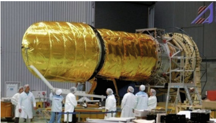
Fig. 14.8 The T-170M telescope model for vibration tests at the Lavochkin Science & Technology Association (Lavochkin Science & Technology Association)
