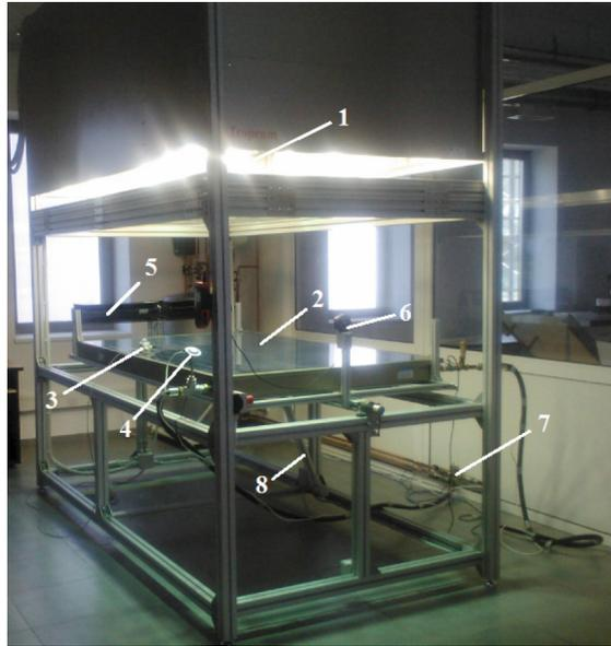
**Fig. 3** Out-door test rig for corrosion/erosion test
