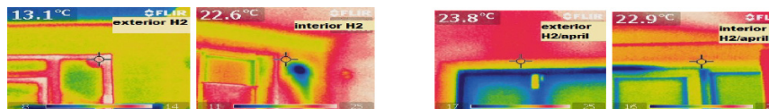
Fig. 4 Analysis of temperature, at wall level in building H2, in November (left), April (right) [6]
