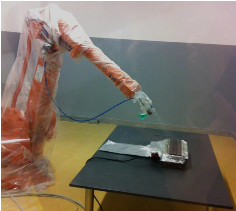
Fig. 1 The industrial robot with six degrees of freedom used in the SPD process
