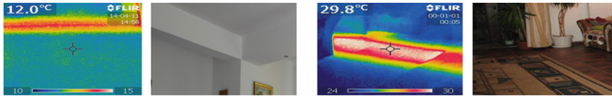
Fig. 6 Checking the routes of heating equipment in the ceiling and floor for building H2 [6]
