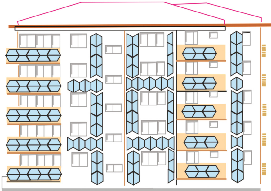
Fig. 19 Horizontally and vertically disposed triangular array units on the façade of a block of flats
