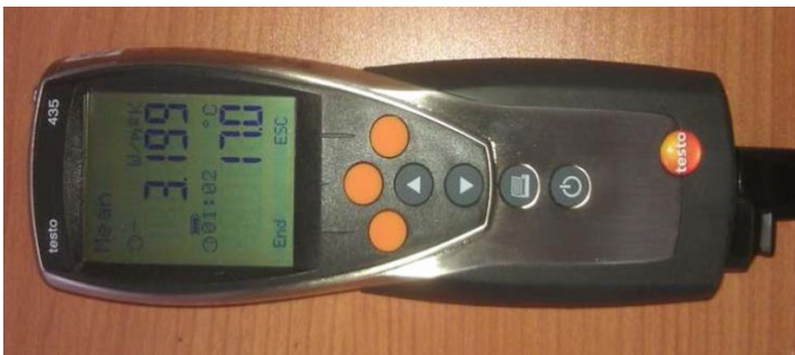
Fig. 3 Digital multimeter and data logger TESTO 435-2
