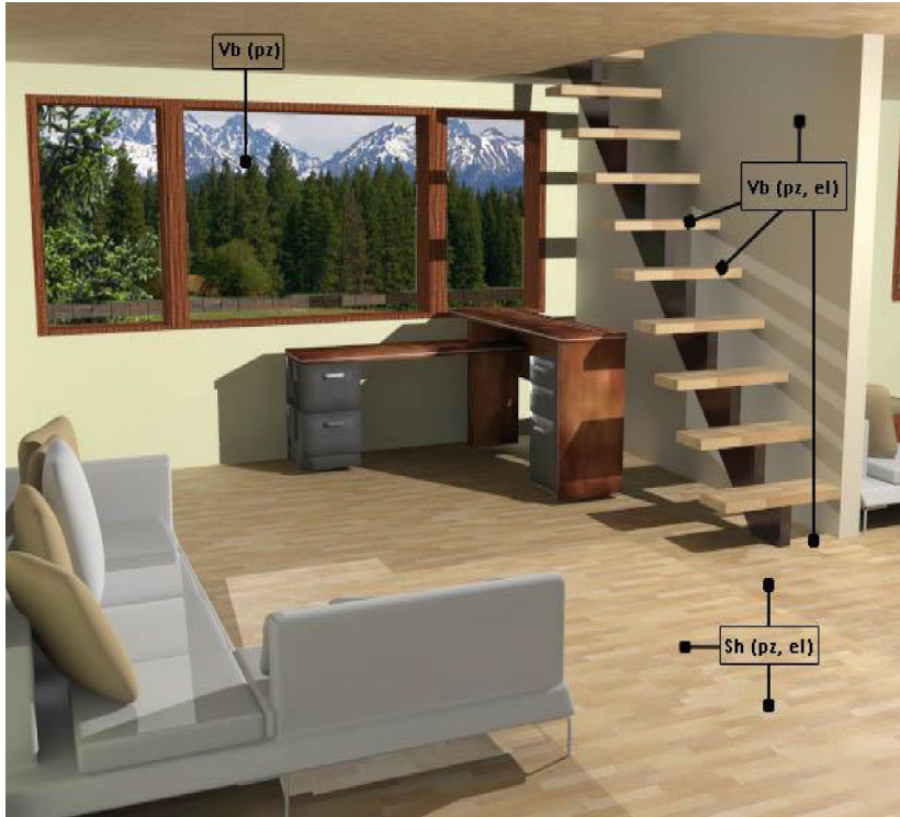
Fig. 3 The harvesting energy microsources in the interior of a building. Vb vibration microsource, sh mechanical shock, pz piezoelectric conversion ( I piezoelectric effect), el electrostrictive conversion on the elastomeric materials
