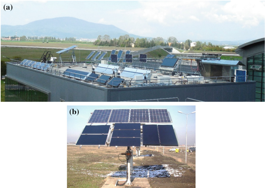
Fig. 8 Outdoor testing rigs in the RES-REC center: a on the roof top of the laboratory L7; b on the ground
