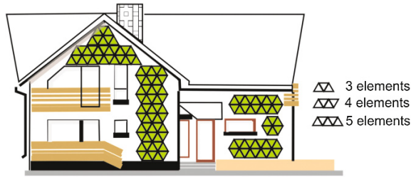
Fig. 15 Horizontally disposed array units with triangular elements on the façade of a residential house
