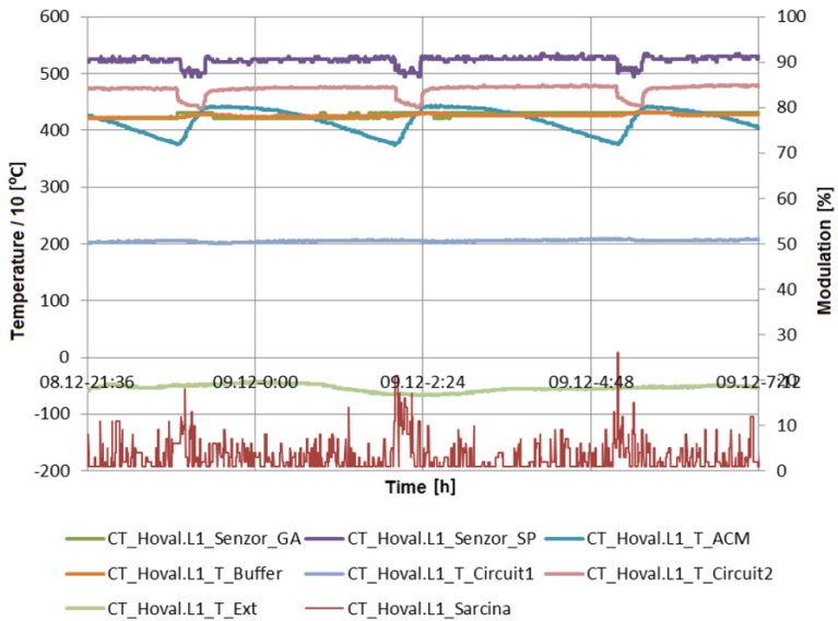
Fig. 10 Monitoring parameters on Hoval radiators
