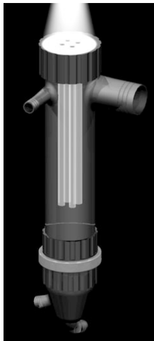
Fig. 5 Scheme of the novel photobioreactor enabling the cultivation of terrestrial cyanobacteria. The reactor is illuminated from the top by LEDs and light is supplemented via roughened glass rods, which are fixed by the lid of the reactor. Light distribution is achieved due to scattering at the boundary of glass/air, thus cyanobacteria growing on the glass surface are supplemented with light. Nutrients and water are provided as aerosol from the connections presented at the upper part of the reactor
