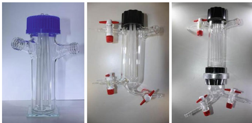
Fig. 6 Different stages of the development of ePBR designs. (Left) First prototype of the ePBR; (Middle) photobioreactor with connectors enabling sampling of liquids and biomass; (Right) photobioreactor in current geometry including a perforated tray for biomass retention
