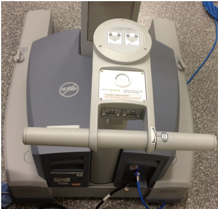
Fig. 3.7 Steering handles of the surgical cart motorized drive. Note the built-in rotary throttle and the brake release clutch on the right and left handles, respectively
