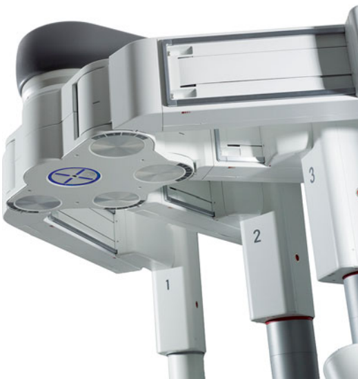
Fig. 15.4 The laser targeting emitter used to assist with docking (Courtesy of Intuitive Surgical, Inc.)
