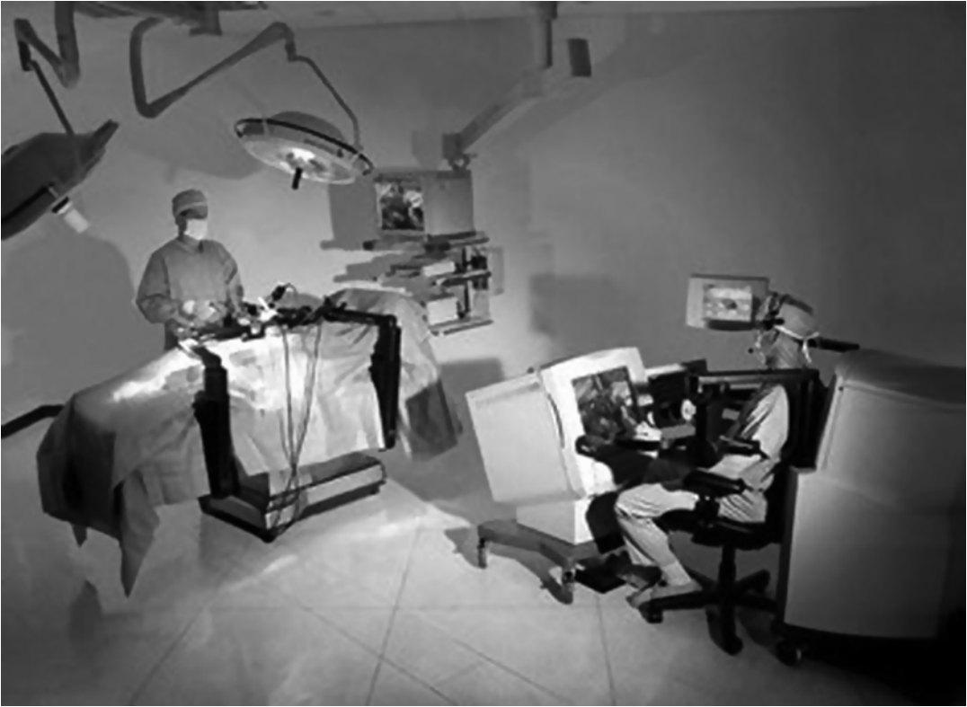
Fig. 1.4 ZEUS Robotic Surgical System (Used with permission from Faust RA, Kant AJ, Lorincz A et al. Robotic endoscopic surgery in a porcine model of the infant neck. J Robotic Surg 2007;1:75–83)
