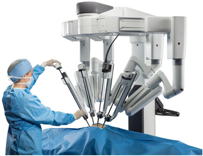
Fig. 15.3 Redesigned arm placement allowing for increased range of motion (Courtesy of Intuitive Surgical, Inc.)
