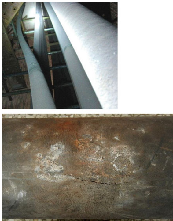
Fig. 10 Creep bending and drum kits of furnace tube
