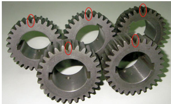
Fig. 4 Configuration of sun gears with different damage seeded
