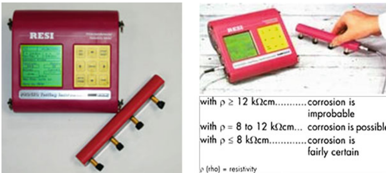
Fig. 6 Resistivity measurement
