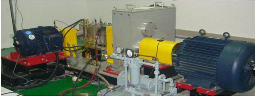
Fig. 2 Helicopter transmission system fault simulation platform
