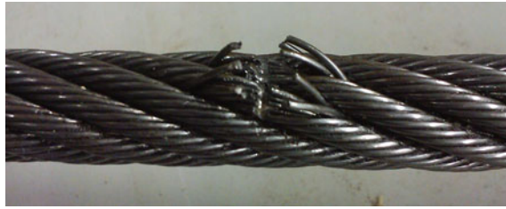
Fig. 12 The broken wire defects in the hoist wire rope
