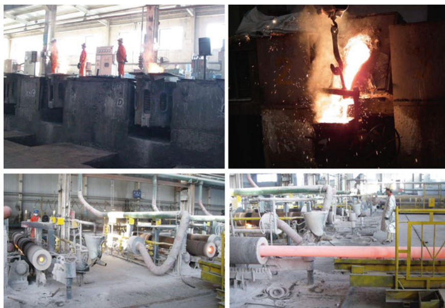
Fig. 3 Typical melting and casting field of furnace tube
