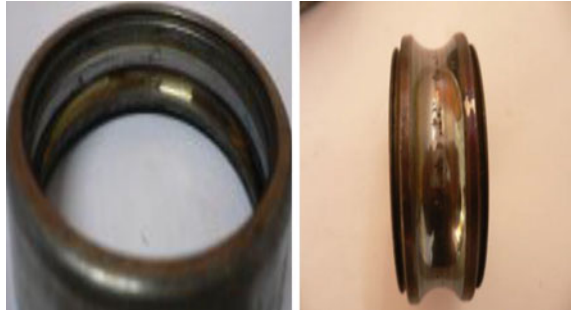
Fig. 12 The photos of failure bearing (inner race fault)
