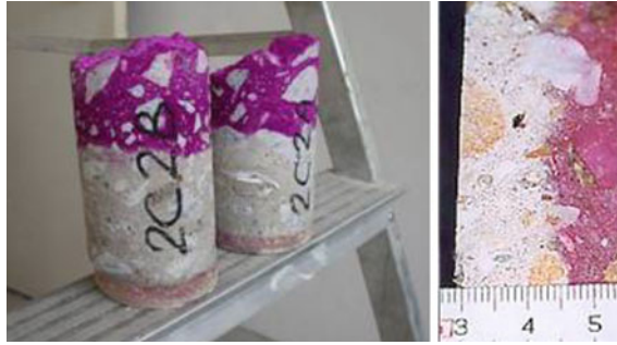
Fig. 5 Carbonation test of concrete cores
