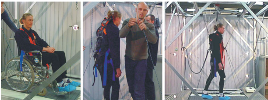
Fig. 1 STRINGMAN—patient attachments supported by lifting-system and wire-attach function (position based force/damping control)
