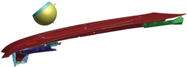
Fig. 7.22 FEA model with head impactor for optimisation
