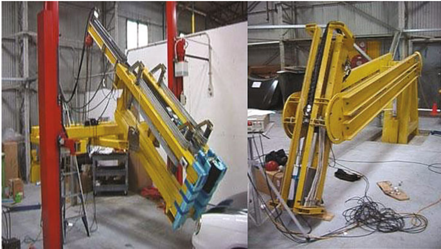
Fig. 7.8 Leg impact and head impact test machines (Centre of automotive safety research 2007)
