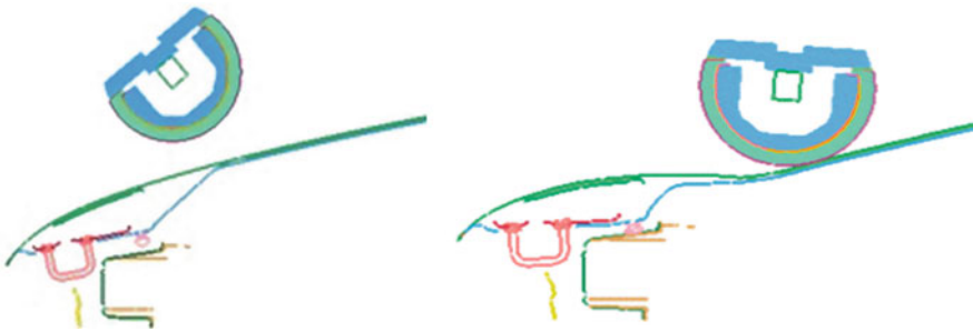
Fig. 7.33 Accelerometer rotation due to impactor rebound
