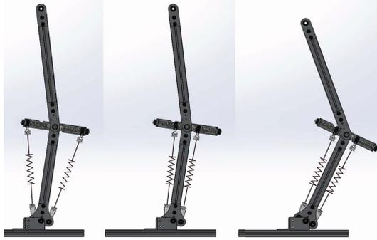
**Fig. 2.** By simultaneously changing the distance between each slider and the joint pivot, the stiffness of the joint can be changed independently of the joint angle without a pneumatic air exchange system (left to center). The neutral position of the joint can be changed with minimal transient effect on stiffness by rotating the control bar (center to right).
