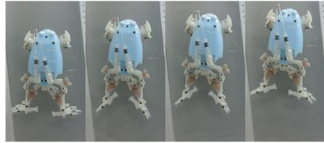
**Fig. 3.** Swimming locomotion by the robot. These are snapshots of swimming locomotion in every 367 msec. The stimulation voltage was 1 V, width of the square pulse was 1 msec, and the pulse period was 21 msec. A sequence of stimulation consisted of 30 pulses and interval between sequences was 1000 msec.
