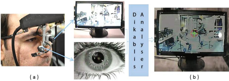
**Fig. 3.** (a) A DIKABLIS eye-tracker with an infrared camera (to capture the participant’s pupil) and an RGB camera (to capture the field video). (b) DIKABLIS analyser merges two recorded videos into a single video, and estimates the participant’s gaze direction on the environment. The participant’s gaze direction is indicated by a green-cross on the screen.
