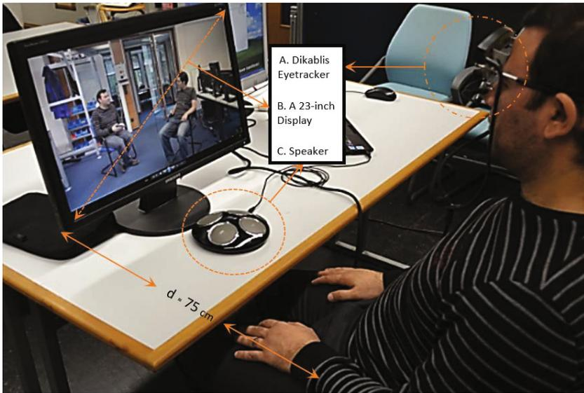
**Fig. 2.** The experiment setup: the participant watched a video while an eye-tracking device recorded the eye-blinking and gaze behaviours
