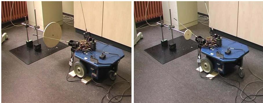
**Fig. 7.** Data acquisition setup for training the distance estimator network of the left antenna. Left: The antenna collide with the large disc (25 cm diameter) at 20 cm distance from the basis of the plastic tube. Right: The antenna collide with the small disc (10 cm diameter) at 10 cm distance from the basis of the plastic tube.
