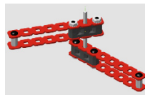
Fig. 2 Unsymmetrical Revolute Joint Design (URJ)
