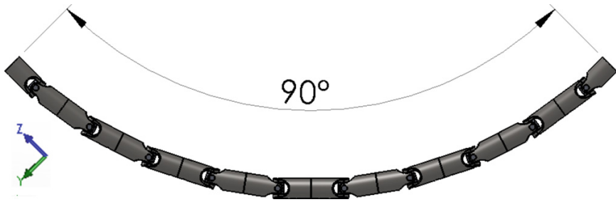
Fig. 3 Basic flexible shaft executing a 90° transmission
