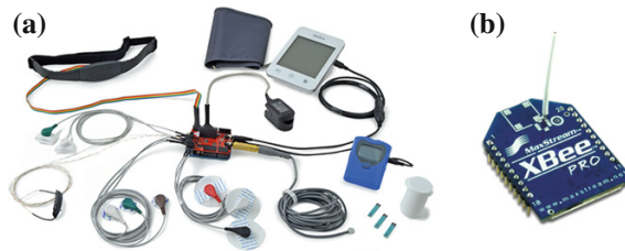
Fig. 1 a The e-health sensor platform; b the MaxStream ® XBee-PRO ™
