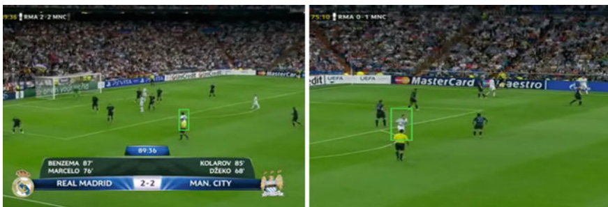
Fig. 5.1 Frames from two different video sequences portraying significant occlusion. The ground truth track of each object is designated in green . Clearly, occlusion renders the tracking problem very difficult. However, certain assumptions about the structuredness of occlusion (e.g., spatial contiguity) can be exploited to alleviate its effect on tracking performance
