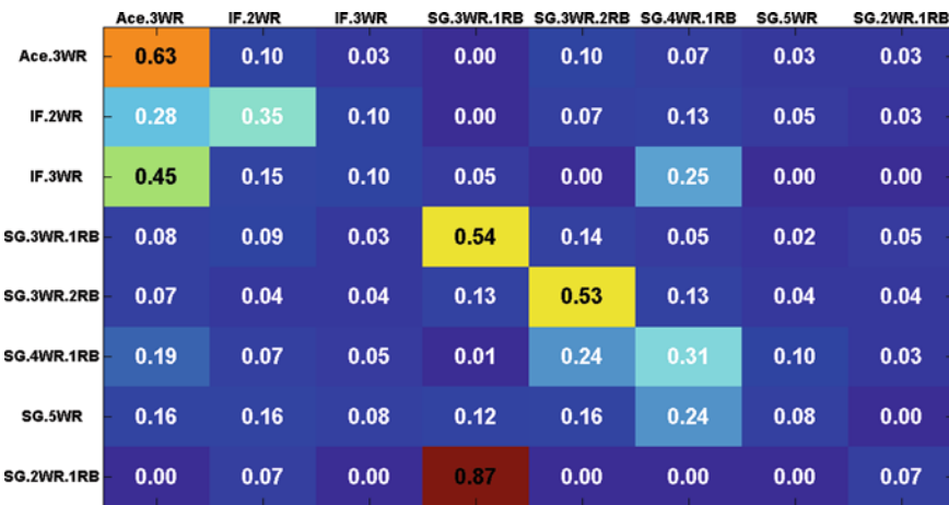
Fig. 13.11 Confusion matrix for the overall classification using all 8 formation classes and structured SVM. The results show an improvement over the linear SVM classification performance
