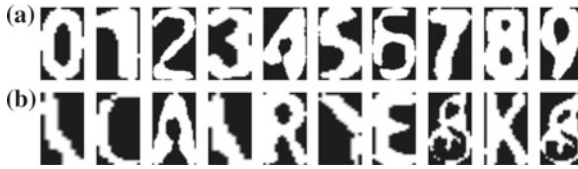
Fig. 14.7 Samples of digit images used to train SVM and ANN in digit detection and recognition tasks: a exemplary digits; b exemplary non-digits
