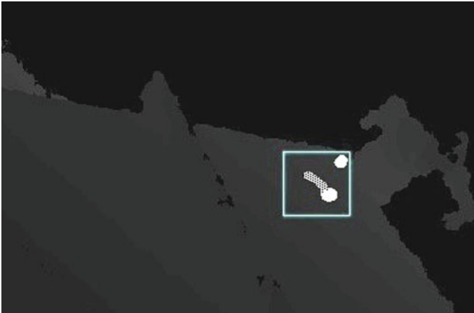
Fig. 3.9 Detection of ball candidates in a depth image. Dotted curve is a 2D trajectory reconstructed based on RGB images. Rectangle is the range of positions where ball can be, which was defined with the trajectory. While segments were candidates, and the closest one was selected as ball
