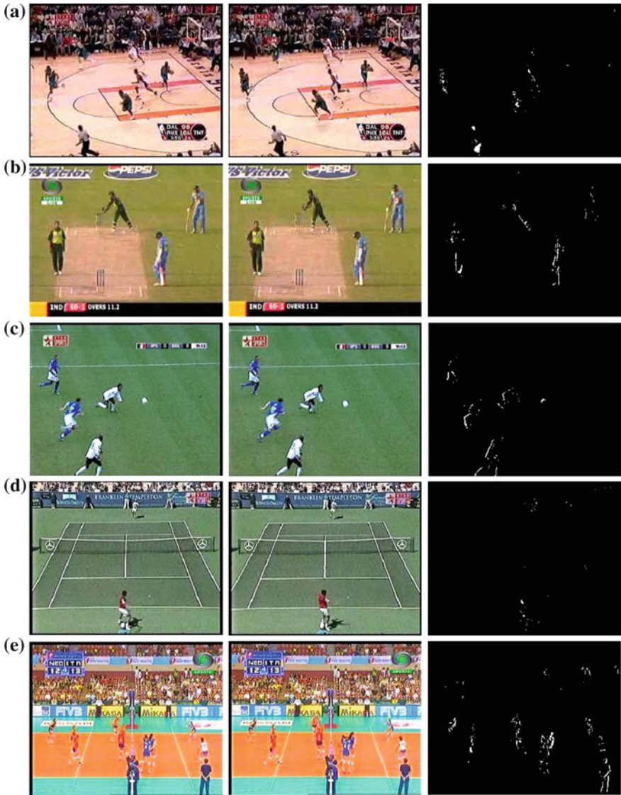
Fig. 11.1 Examples of binary maps for different sports categories. Each row shows two consecutive frames and the corresponding binary map for five different sports, namely, a basketball. b Cricket. c Football. d Tennis. and e Volleyball
