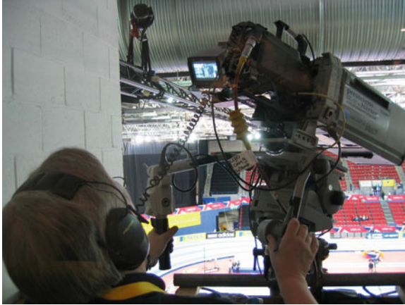
Fig. 1.3 Camera with sensors on lens and pan/tilt mount for virtual graphics overlay
