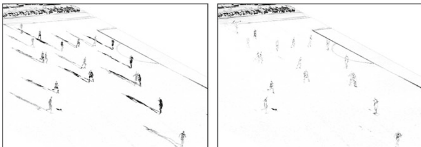
Fig. 7.12 Example for an initial color error when using the ground plane as the geometric proxy. The errors appear at pixels with wrong depth values
