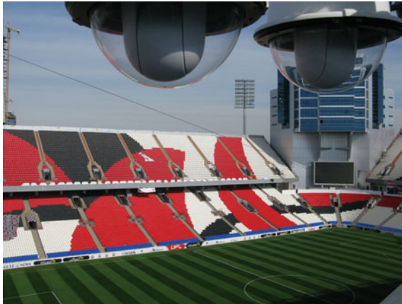
Fig. 1.1 Cameras installed at a football ground for player tracking (picture courtesy of Prozone)
