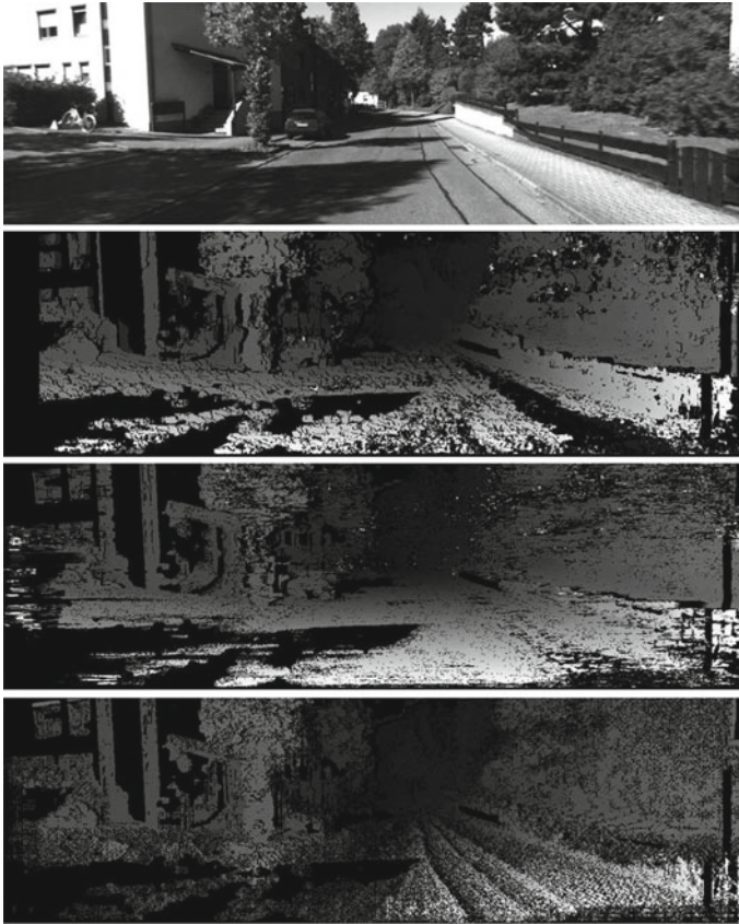
Fig. 5.1 Preliminary experimental results for three algorithms implemented in the target computing architecture. Disparity maps are concerned with frame #66 of the KITTI dataset [10], using a simple x-Sobel filter as prefiltering step. From top to bottom rectified reference image, disparity map computed by the FW implementation, disparity map computed by a modified version of the [5] algorithm using two paths, and disparity maps computed by a modified version of the SGM [13] algorithm using four paths. Additional experimental results are available at this link: http://www.youtube.com/channel/UChkayQwiHJuf3nqMikhxAlw
