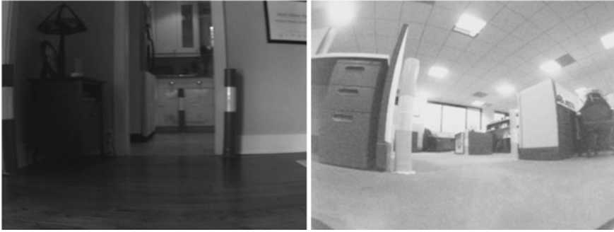
Fig. 2.5 Example images from the SEQ2 ( left ) and SEQ3 ( right ). The reflector beacons are NAV200 fiducials used for ground truth estimation
