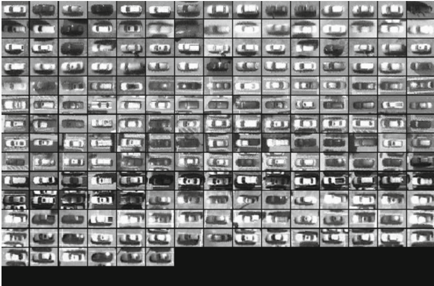
Fig. 9.3 Partial training set for OpenCV’s Viola–Jones style training algorithm for the “aligned” cascade
