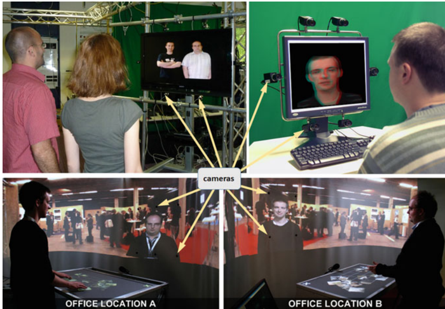
Fig. 6.1 Restoring eye contact by synthesizing a virtual view in between the surrounding camera views
