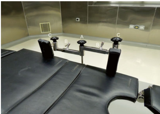
Fig. 15.1 Operating table side support is fixed to the table side rails. (A) Center knob to adjust the arm. (B) Side knob to pull out the inner rod and adjust the length. (C) Outer knob to turn the pad in either direction
