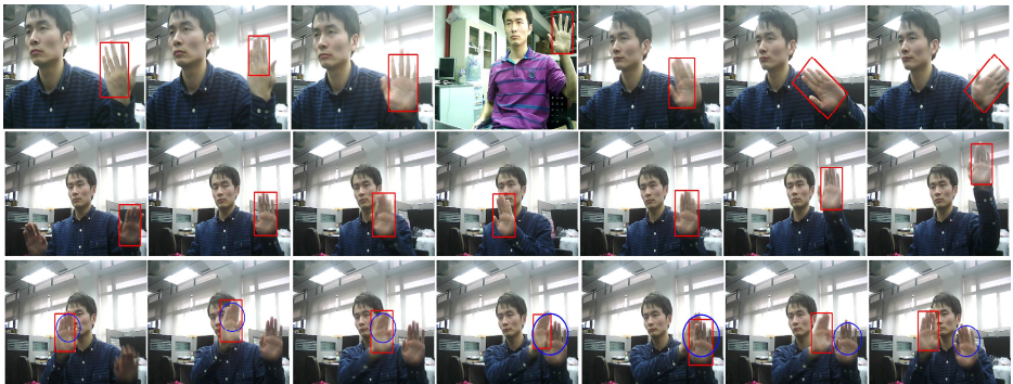
Fig. 7. An illustration of the detection (top) and tracking (middle) performance of our approach and the comparison with TLD (bottom)
