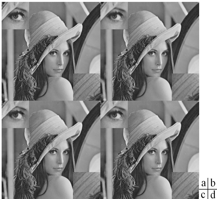
Fig. 2. Comparison of super-resolution results on “Lena” image by different methods: a). Initial high-resolution image; b). Cubic spline interpolation, PSNR=33.5386; c). Conventional fractal coding, PSNR=30.6624; d). The proposed method, PSNR=35.2340
