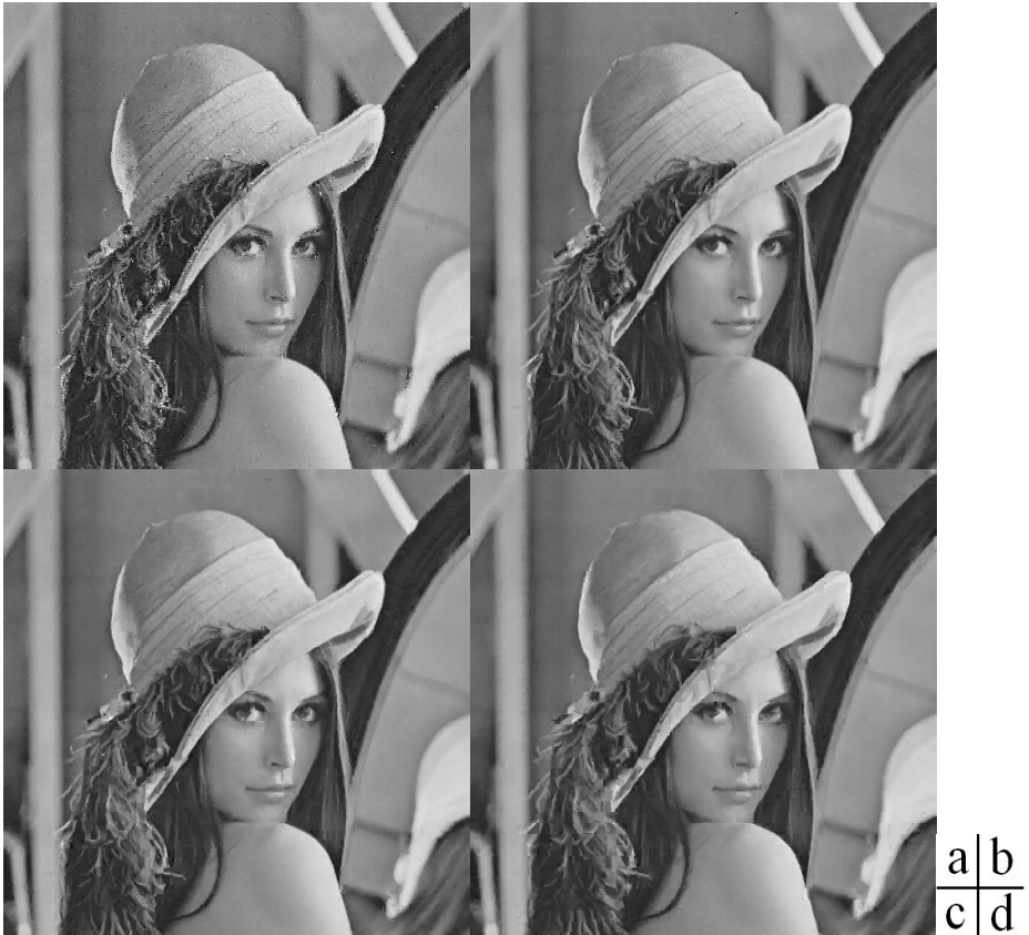
Fig. 1. The reconstructed results by the conventional fractal coding: a). b_r=3 ; b). b_r=4 ; c). b_r=5 ; d). b_r=6
