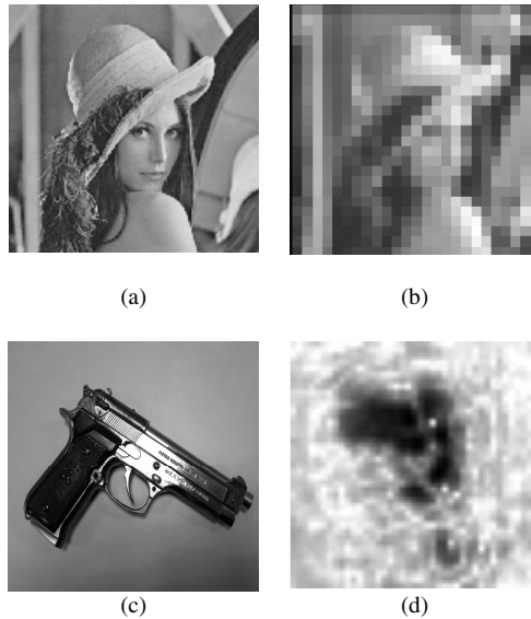
Fig. 1. The original images and the corresponding degenerated images. (a) The original Lena image; (b) Noise version of Lena image with noise level 0.01; (c) The imaging target ; (d) MMW image.
