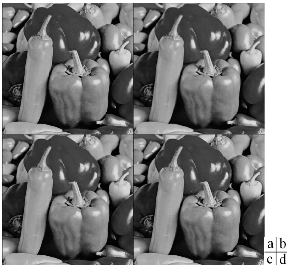
Fig. 4. Comparison of super-resolution results on “Pepper” image by different methods: a). Initial high-resolution image; b). Cubic spline interpolation, PSNR=32.0085; c). Conventional fractal coding, PSNR=30.6253; d). The proposed method, PSNR=34.1000
