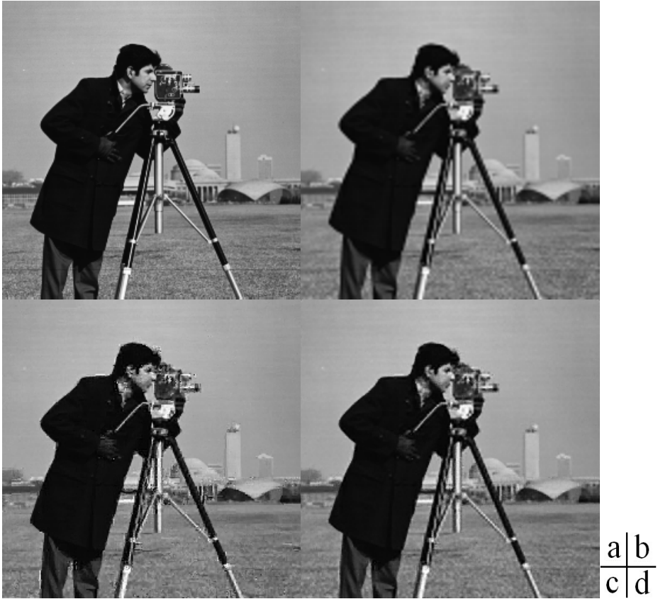
Fig. 3. Comparison of super-resolution results on “Cameraman” image by different methods: a). Initial high-resolution image; b). Cubic spline interpolation, PSNR=26.5226; c). Conventional fractal coding, PSNR=24.8891; d). The proposed method, PSNR=27.2482
