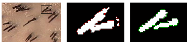
Fig. 5. Image segmentation. Left image is the original image, middle image is pseudo-cross phenomena, and left image shows the correct result with our proposed algorithm.
