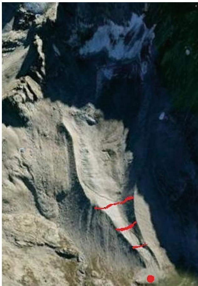
Fig. 33.3 The GPS kinematical traces made during 2011–2012–2013 in the snout position of Capra Glacier. The red dot shows the positioning of fixed position. Scale 1:10,000
