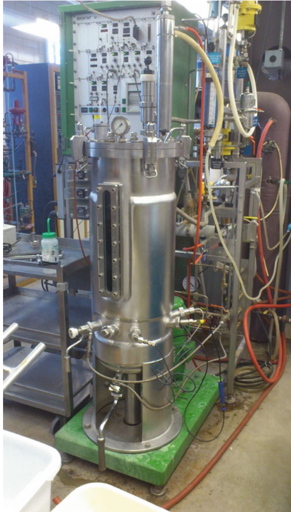
Fig. 2.4 Cultivation of bacteria for biocement production in 50 L fermentor(photo taken at the Fermentation Facility, Iowa State University,USA)
