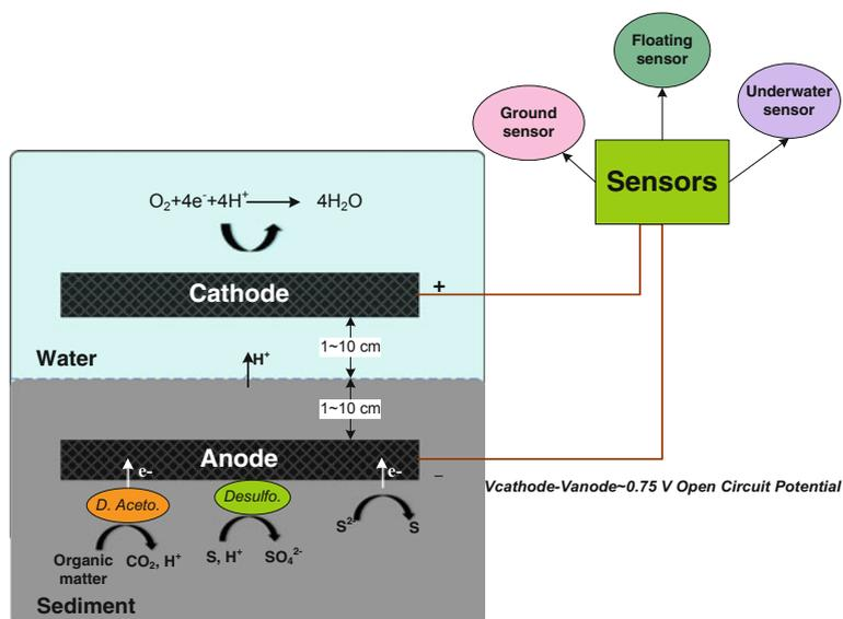
**Fig. 18.5** Schematic representation of fundamental principle of the mediator less sediment MFCs used to provide energy for on-site sensors. Microorganisms colonizing the anode are most similar to *Desulfuromonas acetoxidans* (*D. Aceto.*), which could oxidize acetate in sediment and transfer electrons to the anode. *Desulfo.* represents the species in the *Desulfobulbus* or *Desulfucapsa* genera, which could oxidize anode generated  $S_0$  to  $SO_4^{2-}$
