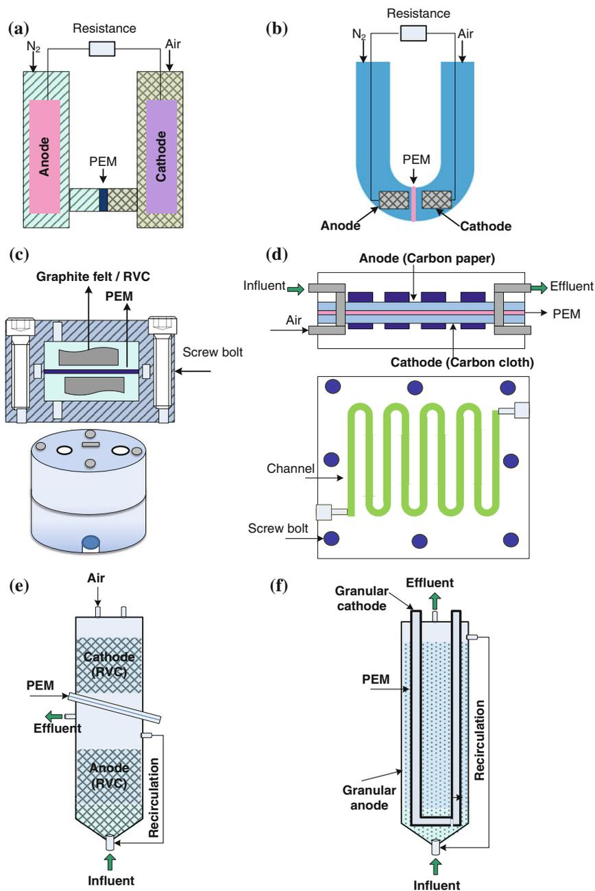
**Fig. 18.2** Schematics of typical two-chamber MFCs: **a** H-type MFC with PEM or salt bridge; **b** U-shaped MFC; **c** Mini-MFC; **d** Flat plate MFC; **e**, **f** Up flow MFC with cylindrical shape
