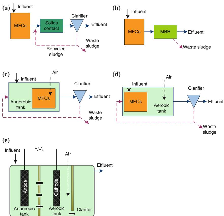
**Fig. 18.6** Schematic diagram of MFCs combined wastewater treatment process: **a, b** MFC combined with a solids contact tank or a MBR; **c, d** MFC submerged into an anaerobic or aerobic tank of existing wastewater treatment process; **e** a decentralized wastewater treatment based on A/O system
