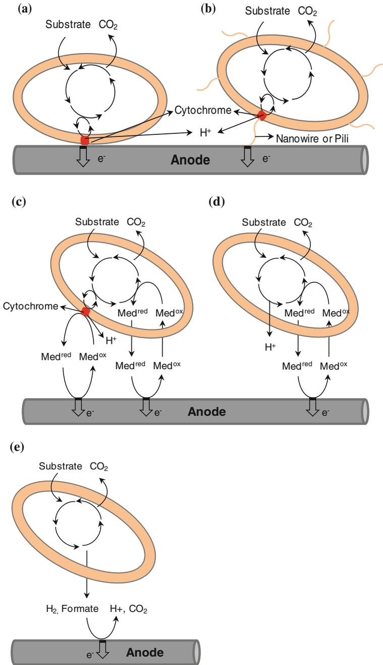
**Fig. 18.4** Electron transfer mechanism of exoelectrogens: Direct electron transfer by **a** attachment of cell membrane or **b** nanowire; Indirect electron transfer by **c** exogenous mediators, **d** endogenous secondary metabolites or **e** primary metabolites
