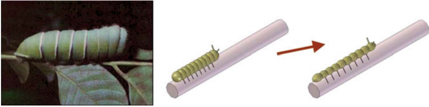
Fig. 11.6 The ability of a worm to shrink and extend its own body to propel itself forward has inspired the creation of artificial counterparts that mimic this behavior (Balaguer et al. 2005). (Images provided courtesy of Springer)
