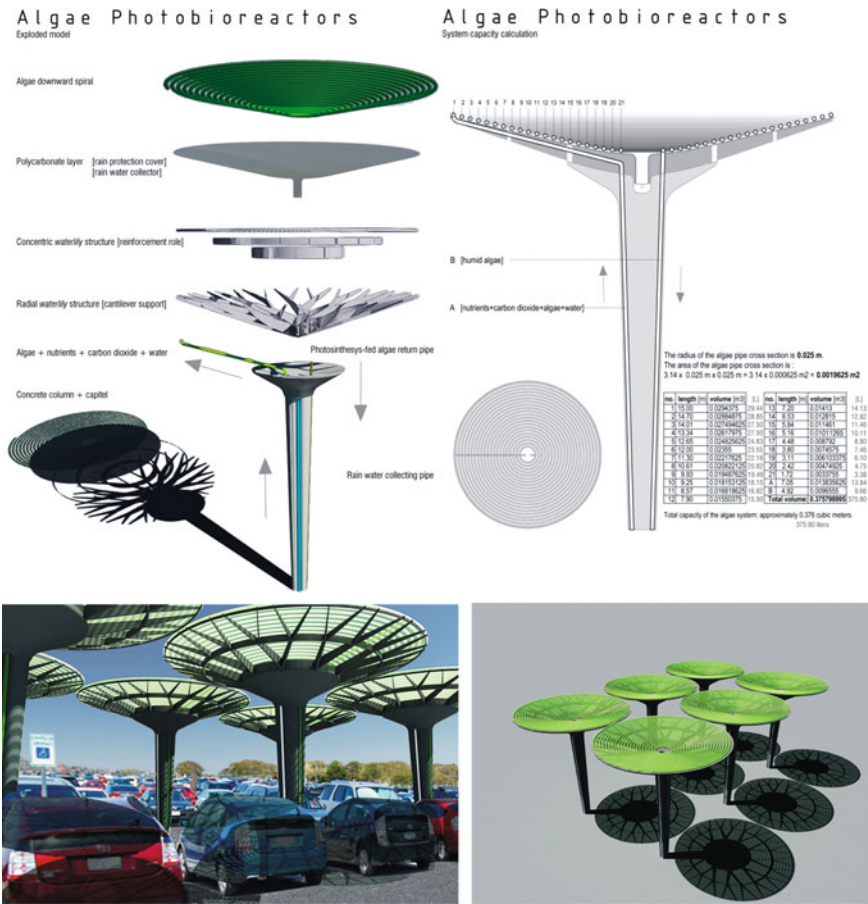
Fig. 7.8 Photo-biorreactor integrated in the street furniture, canopies (Design by R. Cervera and J. Pioz)
