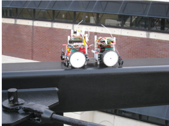
Fig. 11.3 A mobile sensor prototype (developed by researchers at the Georgia Institute of Technology, USA) is crawling on a steel pedestrian bridge. (Photo courtesy of Prof. Yang Wang, Georgia Institute of Technology, USA)
