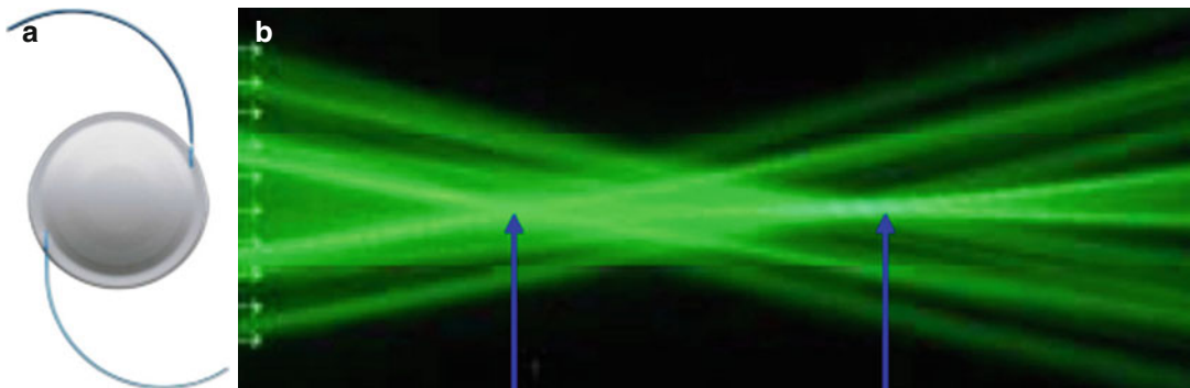
Fig. 2.22 The display of focal points (b) of the AMO ReZoom lens (a)
