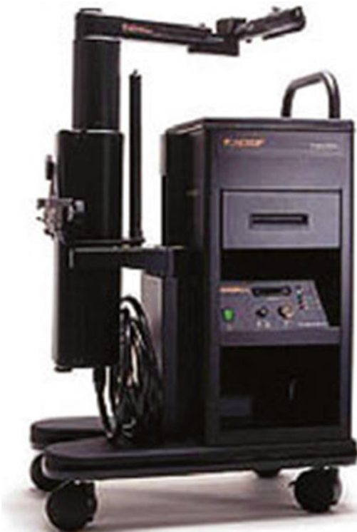
Fig. 1.6 AESOP (Automated Endoscopic System for Optimal Positioning). With permission from M.L. Lorentziadis A Short History of the Invasion of Robots in Surgery . Hellenic Journal of Surgery (2014) 86:3, 117–121. © Springer
