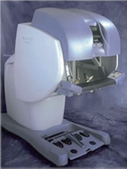
Fig. 1.7 da Vinci surgical system console. With permission from Ilya A. Volfson, Jeffrey A. Stock. History of Robotic Surgery. In: Jeffrey A. Stock MD, Michael P. Esposito MD, Vincent J. Lanteri MD, David M. Albala MD, eds. Current Clinical Urology: Urologic Robotic Surgery. Springer, New York 2008: pp 3–25. © Springer
