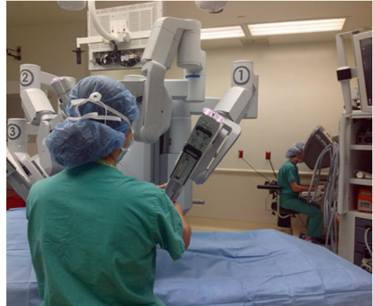
Fig. 9.2 The console surgeon is immersed in the operation, while the bedside surgeon must ensure the safe interaction between the robot and the patient
