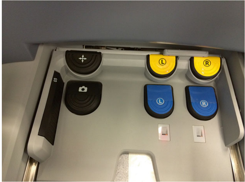
Fig. 3.6 Foot switch panel
