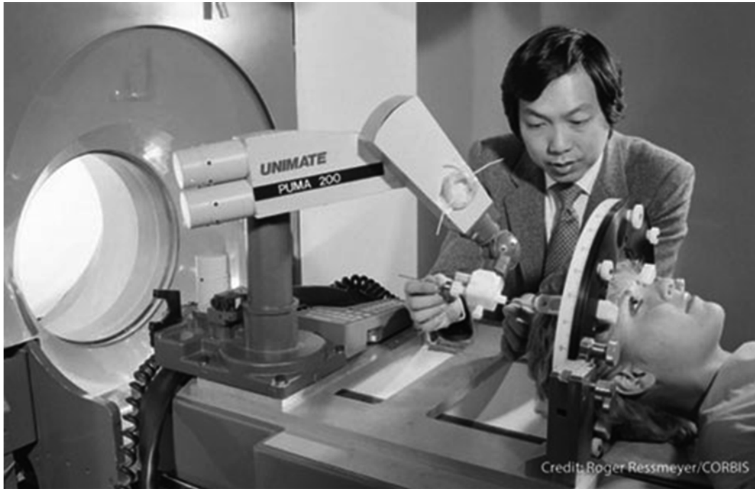
Fig. 1.2 Puma 200 robot. With permission from M.L. Lorentziadis A Short History of the Invasion of Robots in Surgery. Hellenic Journal of Surgery (2014) 86:3, 117–121. © Springer
