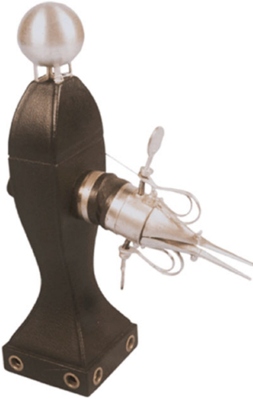
Fig. 2.3 The Lichtleiter created by Austrian Philipp Bozzini in 1805, the first illuminated scope which consisted of a rudimentary viewing tube, a series of mirrors, and a candle as a light source
