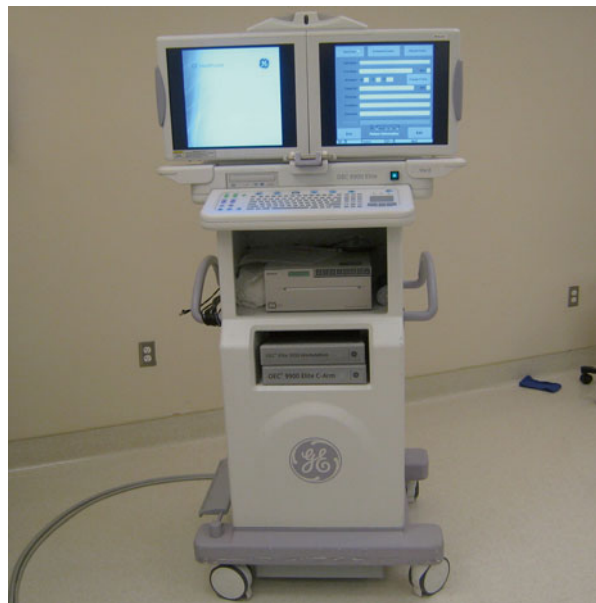
Fig. 1.5 The monitor console in a mobile fluoroscopic imaging system is mounted on wheels and can be moved together with the mobile C-arm from room to room
