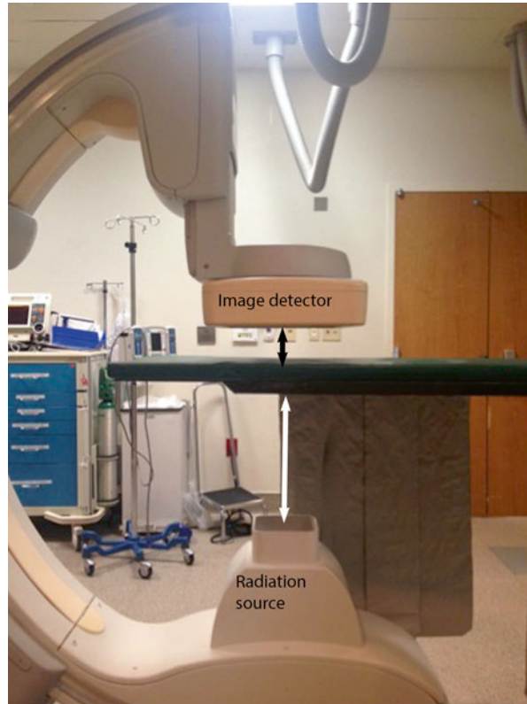
Fig. 4.4 Flat panel fluoroscopic unit illustrating minimization of distance from the image detector to position of the patient on the procedural table ( black arrow ) and maximizing the distance from the radiation source to the patient on the procedural table ( white arrow )
