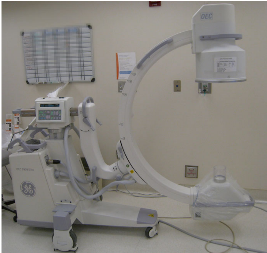
Fig. 1.2 The portable C-arm of a mobile fluoroscopic imaging system. The radiographer manually positions the C-arm over the area of intervention
