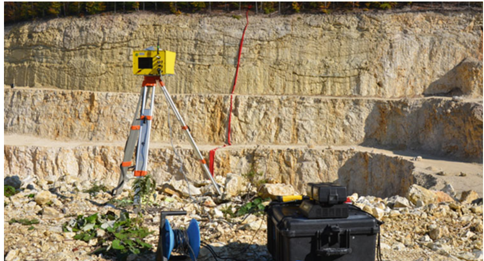
Fig. 34.1 Tripod mounted instrument, scanning a 65 m height slope. Light-colored lime —and marlstone, complex geological features and different rock face conditions due to ongoing quarrying complicate the rock classification
