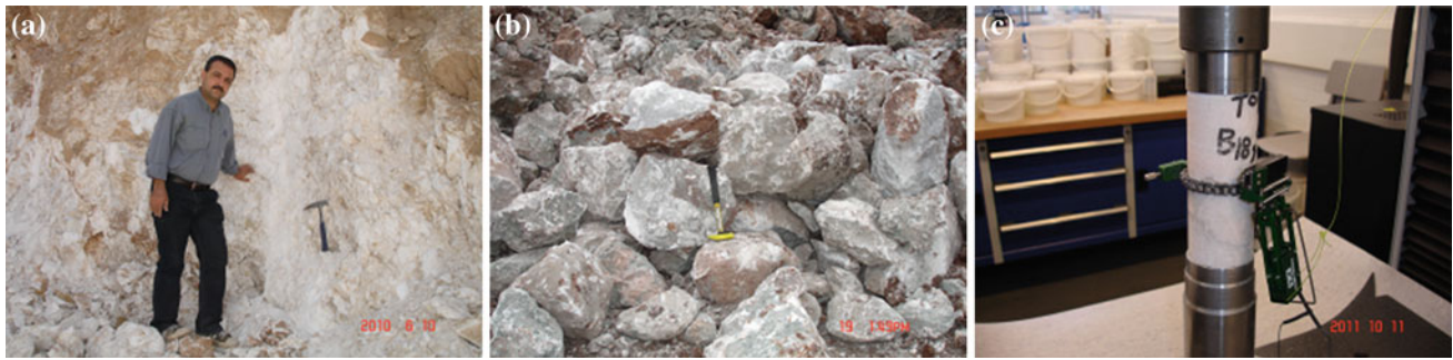
Fig. 139.2 a Gypsum outcrop, Bazyan/Iraq b Bantycoc Mine/UK gypsum blocks c The extensometer in the mid-length of a cylinder
