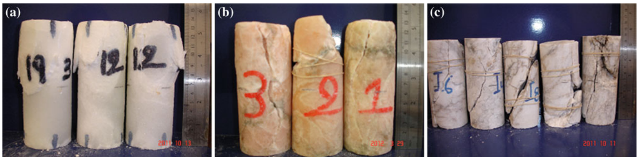
Fig. 139.3 The failed cylinders after short-term loading: a The white/Bantycoc gypsum. b The pink/Bantycoc gypsum. c The Iraqi gypsum
