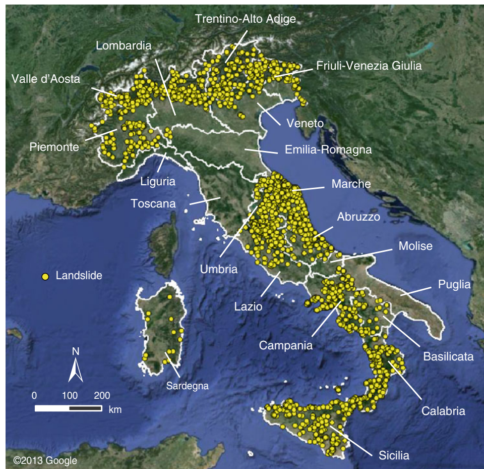
Fig. 280.1 Map showing the location of 2408 rainfall-induced shallow landslides (yellow dots) in Italy between 1996 and 2012. The map shows the 20 Italian administrative regions
