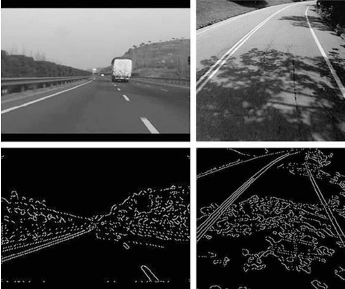
Fig. 70.2 Original image and image handled by Gabor filter. We can see that under the condition of not changing any parameter, Gabor filter can still get good effect of edge detection
