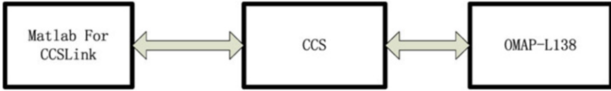
Fig. 91.4 The connection between CCSLink, CCS and DSP
