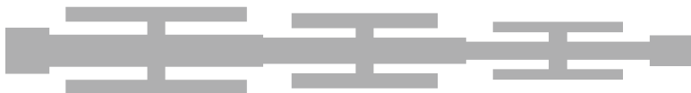
Fig. 9 Geometry of an exemplary matching transformer composed by cascading three SWRS sections of Fig. 7
