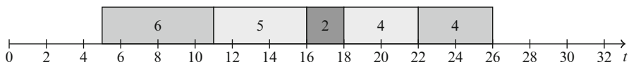
Fig. 3 All the jobs are shifted left by \min\{ES, DT_j\} = 2 units processing time
