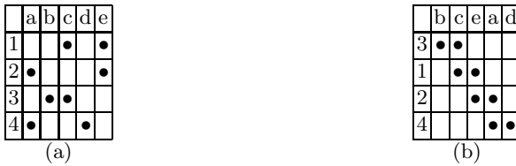
Fig. 1. Banding Example: (a) raw data (b) rearrangement of columns and rows to reveal a banding
