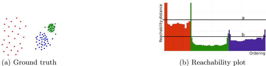
Fig. 2. The two lines in the reachability plot represent two different thresholds. Using the upper line that represents a higher threshold, leads to two clusters, where the blue and green areas are recognized as a single cluster and the red cluster is correctly recognized. The lower line corresponds to a lower threshold recognizes only the blue and green clusters.
