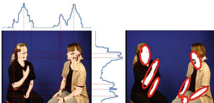
Fig. 1. Histogram of skin color points (left) and examples of ellipses approximating the skin areas in given image (right) (Color figure online)
