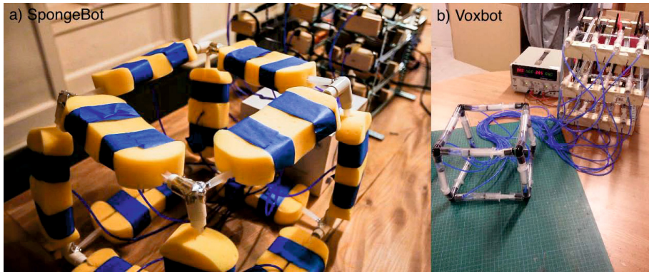
Fig. 1. Development stages of the robot cube and servo control system. Left: SpongeBot and original servo control system. Right: Voxbot and smaller updated servo controller.
