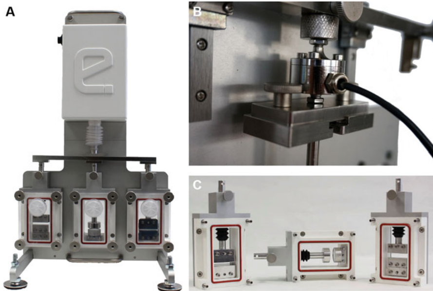
Fig. 6 TC-3 bioreactor by Ebers Medical. (a) The system can be equipped with three independent chambers. Different chambers for the application of (b) hydrostatic pressure or (c) tension, compression and tension combined with compression are available. Pictures kindly provided by Ebers Medical
