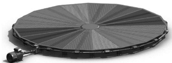
Fig. 2 CAD model of the omnidirectional floor
