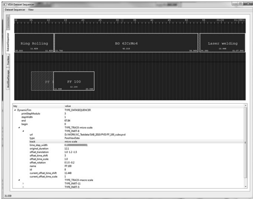
Fig. 6 The employed interaction metaphor on top of the Dataset Sequencer : Intuitive user interface for manipulation of the chronological configuration of a visualization scenario
