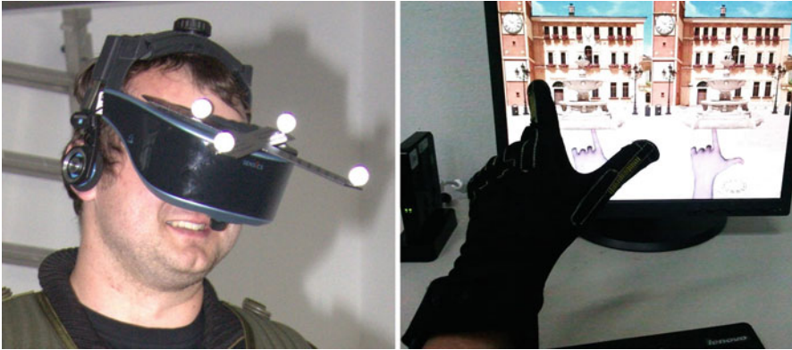
Fig. 3 Head mounted display with attached infrared markers ( left ); Data glove and representation in a virtual environment ( right )
