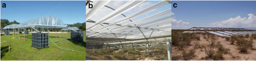
Fig. 4 Experimental designs to study the effects of precipitation manipulation: (a) closed shelters after Jongen et al. (2013b); (b) throughfall shelters, after Yahdjian and Sala (2002), picture from K. Tielbörger; and (c) movable shelters, after Báez et al. (2013), picture from S. Collins
