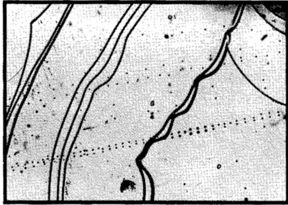
Fig. 2.31 Interaction between dislocations in parallel glide planes ( 180\times ). Reprinted with permission from [81]. Copyright 1960, AIP Publishing LLC
