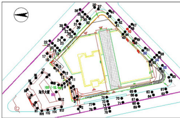
Fig. 4.2 Pit settlement monitoring point layout
